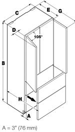
$\begin{array}{l} A = 3" \ (76 \ mm) \\ B = 79^{13/16"} \ (2027 \ mm) \\ C = 35^{13/16"} \ (910 \ mm) \\ D = 3" \ (76 \ mm) \\ E = 24" \ (610 \ mm) \\ G = 42^{7/16"} \ (1078 \ mm) \\ H = 37^{1/8"} \ (943 \ mm) \end{array}$
